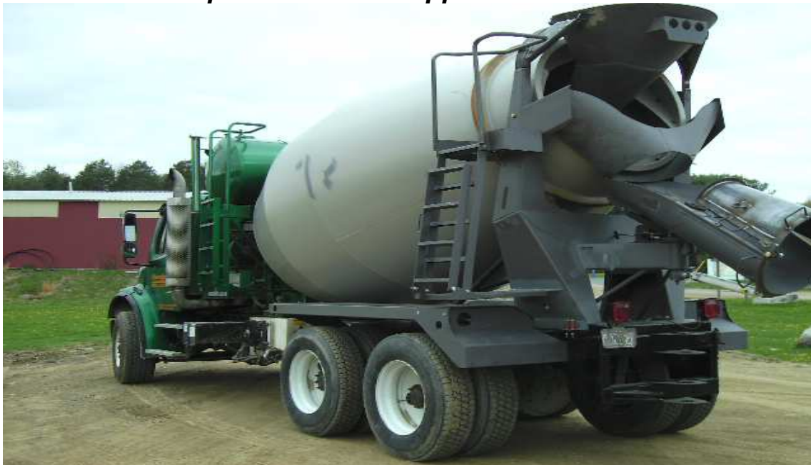
This truck was rollover, we replaced drum and complete rear pedestal with hoppers and chutes
