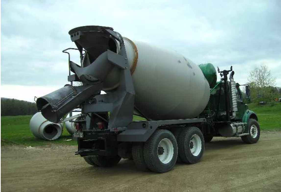
This truck was rollover, we replaced drum and complete rear pedestal with hoppers and chutes
