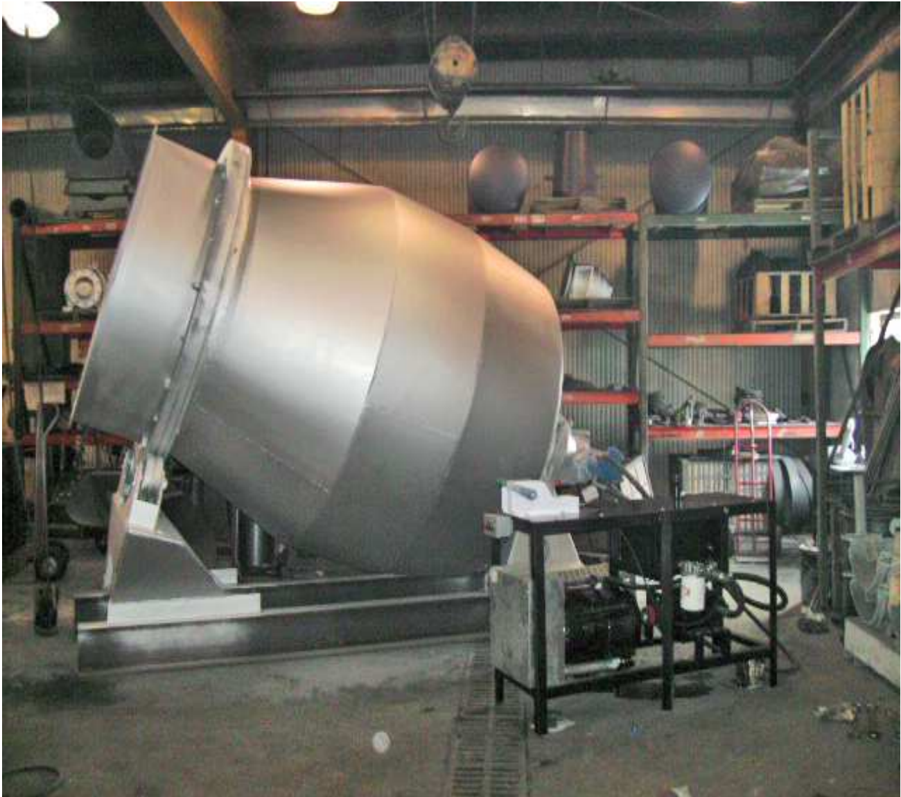
WASTE RECYCLING UNIT with TURNING STATION SIDE VIEW - OVERALL LENGTH 12FT
