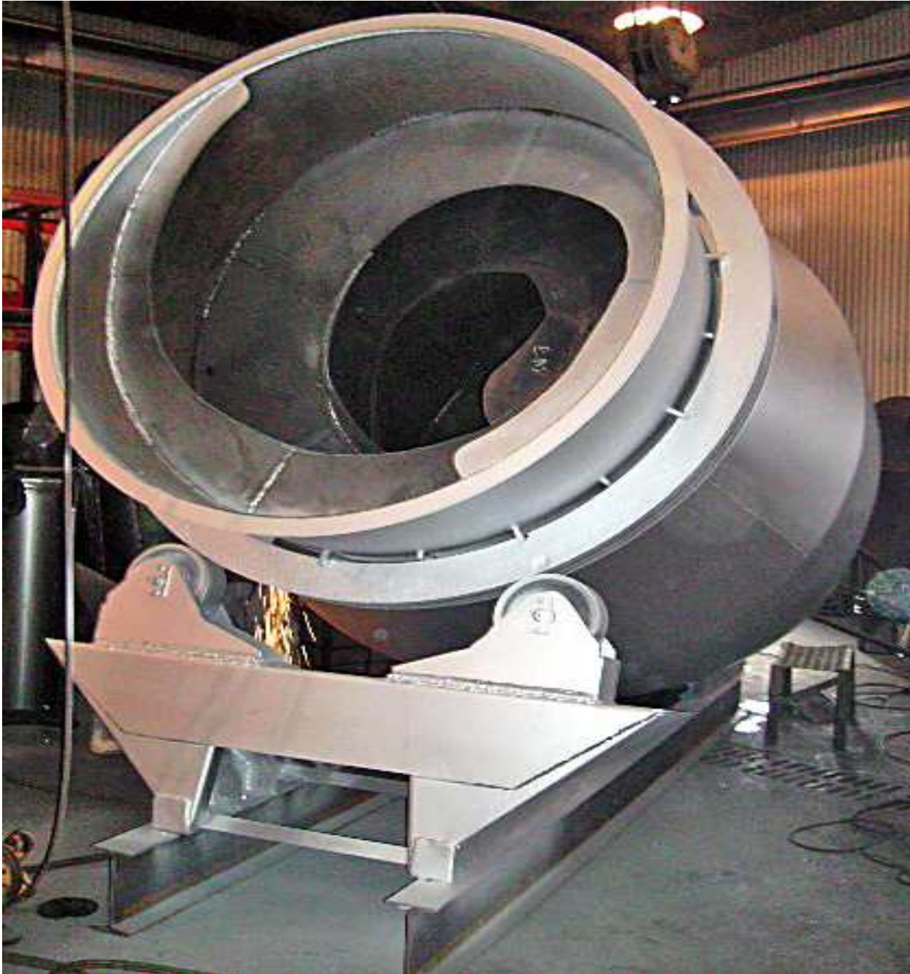
WASTE RECYCLING UNIT 4-5 YARD DRUM - REAR VIEW TAIL OPENING IS 62"
